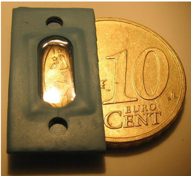
Fig. 10. The LTCC-glass transparent microfluidic chamber.
